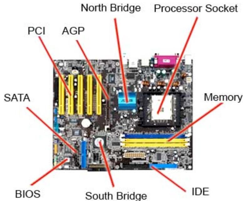
A motherboard by itself is useless, but a computer has to have one to operate. The motherboard's main job is to hold the computer's microprocessor chip and let everything else connect to it. Everything that runs the computer or enhances its performance is either part of the motherboard or plugs into it via a slot or port.
